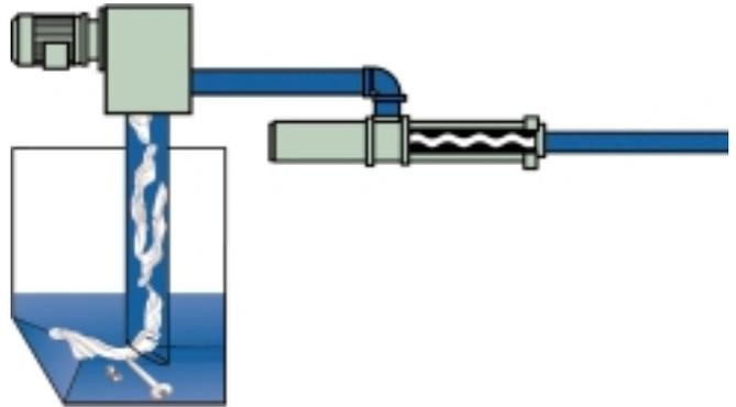
Low suction velocities ensure foreign object damage is eliminated, unlike pumping stations with submersible pumps. Any large objects remain in the sump for periodic removal, avoiding any pump damage.
