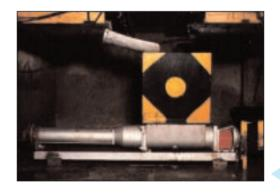
A custom-built W082 is speeding up waste disposal at a Scottish tannery. Previously the 'fleshings' were shovelled manually from the processing area to a skip, this method was highly labour intensive. The cast iron W range pump with large auger and hopper were specially modified in order to handle this difficult material. The fleshings waste is gravity fed into the hopper, then pumped at 5.5m³/h at a pressure of 3 bar, along 30m of pipe direct to an outside skip for disposal.
